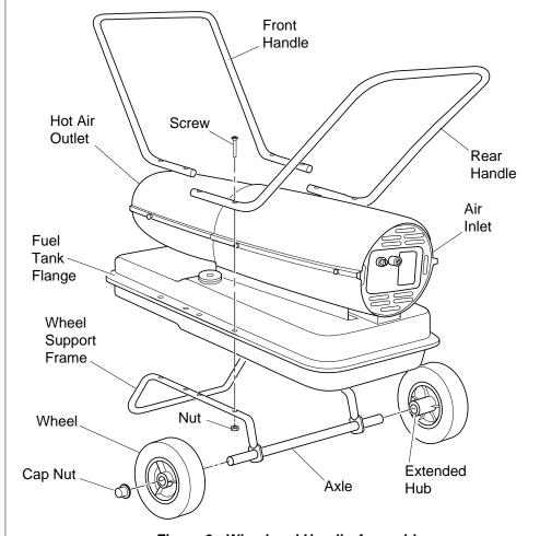
Figure 3 - Wheel and Handle Assembly
